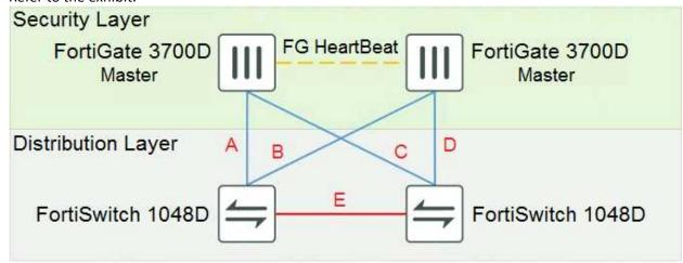
The exhibit shows a full-mesh topology between FortiGate and FortiSwitch devices. To deploy this configuration, two requirements must be met:
