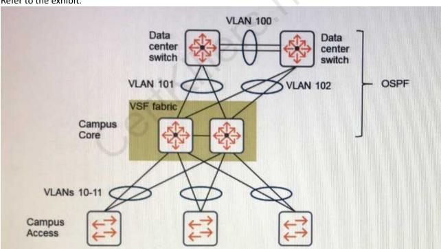
The customer requires fast failover if any one link or core device fails. Which additional technology should the
