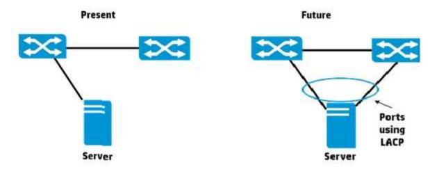
The exhibit shows the physical connection between two HP Comware switches and a server The network administrator is concerned about redundancy and wants to implement a solution like that shown on the right side of the exhibit. The administrator plans to use an LACP link aggregation with both links active. What must the administrator do first?
