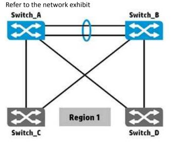
Switch\_A and Switch\_B are HP Comware switches currently in the same Multiple Spanning Tree
