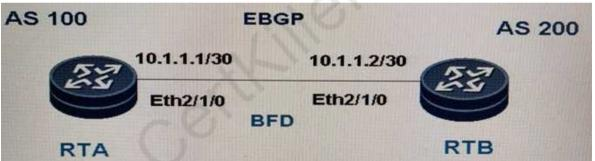
As shown in the figure, RTA and have one BGP session. To detect fault fast, the BFD for BGP feature needs to be configured on RTA and RTB. BGP-related configurations are as follows:
