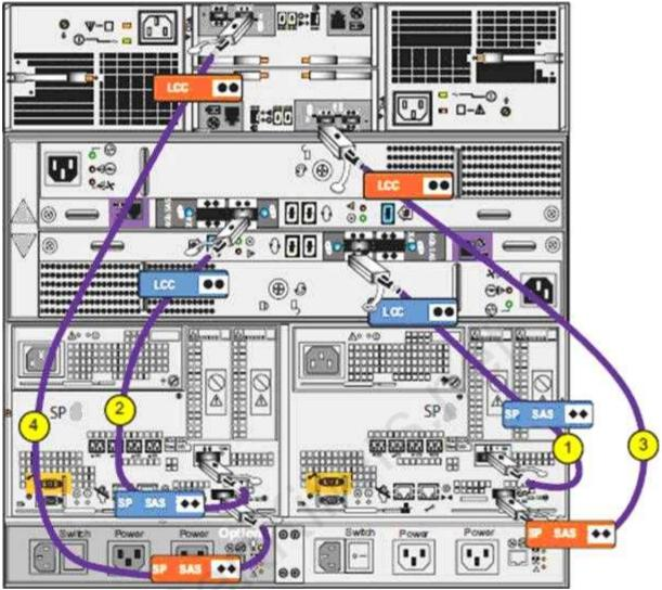
Which DAE and components does cable 1 connect?
