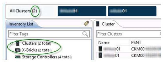
Note: With time, additional clusters can be added to a deployed XMS. In addition, a cluster can be easily moved from one XMS to another. All management interfaces (GUI/CLI/REST) offer inherent multi-cluster management capabilities. Multiple cluster management is supported from version 4.0 and up.
