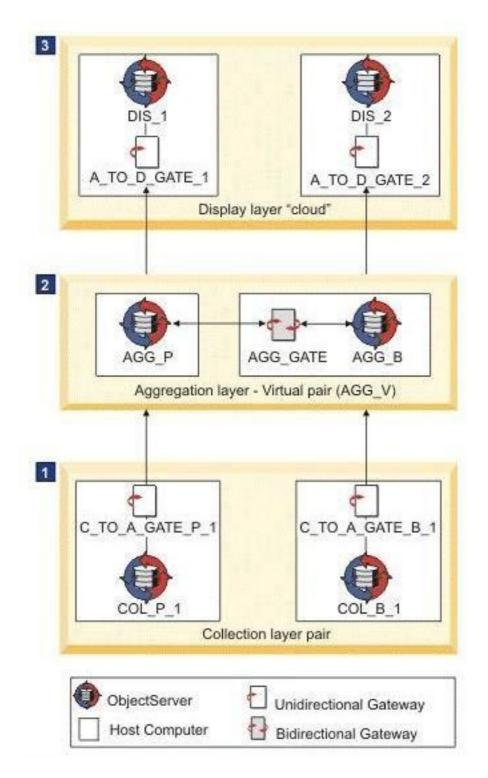
Widgetcom has deployed this 3-tier standard multi-tier architecture deployment of IBM Tivoli Netcool/OMNIbus V7.4 (Netcool/OMNIbus) using the best practice configuration that ships withthe product: The Netcool/OMNIbus administrator wants to examine the contents of a custom table on both AGG\_P and AGG\_B to verify that data is flowing correctly between the primary and backup Aggregation ObjectServers Which two commands can be used to examine the contents of this table? (Choose two)
