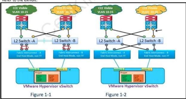
Refer to the exhibit. Which option describes Cisco Unified CCE on the UCS B Fabric Interconnection pair to the upstream network connectivity?
