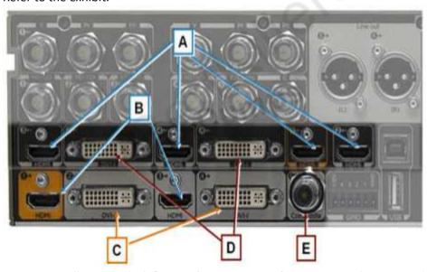
You are installing a high-definition (720p or 1080p) monitor on the Cisco TelePresence Codec C90. Which of the outputs that are represented by letters in the exhibit should you use?
