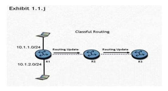
Routers R1 " R2, and R3 are running a classful routing protocol between them. Assuming that router R1 advertises all directly connected networks, how will these networks be represented in router R3's routing table?
