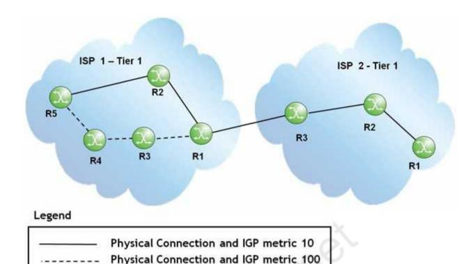
Assuming a full iBGP mesh in ISP 1, how does router R1 in ISP 1 handle a BGP update received from ISP 2?
