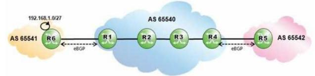
AS 65540 is using MPLS to provide BGP shortcuts for its iBGP routing. Which routers must be configured with the "configure router bgp igp-shortcuts rsvp-te" command?
