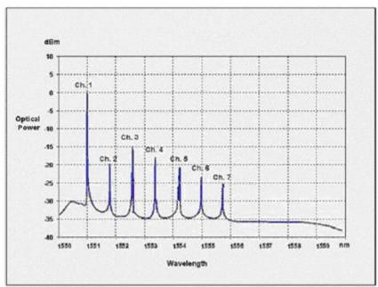
The graph represents optical signal power versus wavelength measurement from 1550nm to 1560nm. The spectral characteristic in the 1558nm to 1559nm range is commonly known as:
