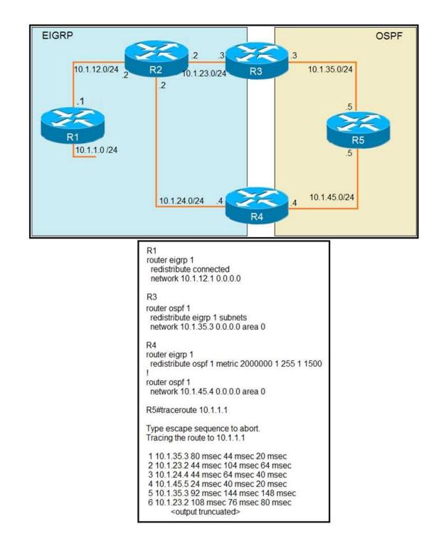
The output of the trace route from R5 shows a loop in the network. Which configuration
