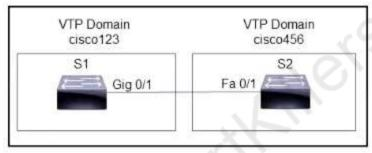
Dynamic trunk negotiation fails between S1 and S2 Which cause of the problem is true?
