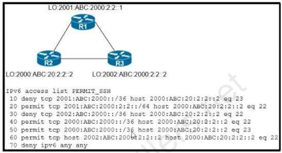
Which sequence number must be moved to the top of the ACL to enable access from R3 to R2?
