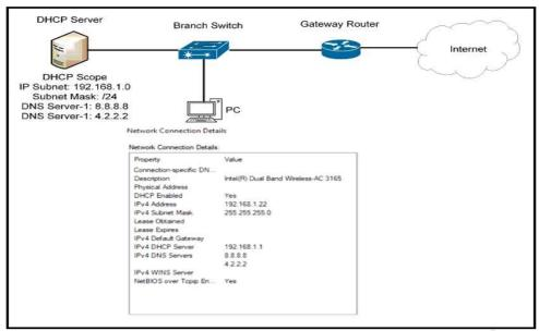
The PC is unable to connect to the Internet. You have determined that the DHCP server has not issued a default gateway to the PC. Which configuration mechanism will resolve this issue?
