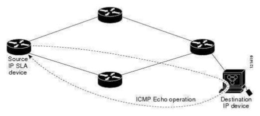
The IP SLAs ICMP Echo operation conforms to the same IETF specifications for ICMP ping testing and the two methods result in the same response times.
