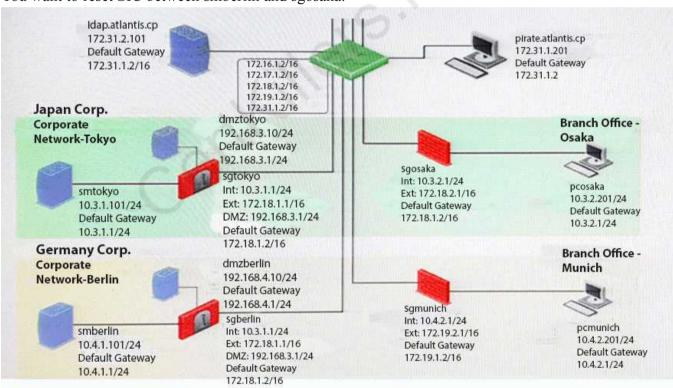
In SmartDashboard, you choose sgosaka, Communication, Reset. On sgosaka, you start cpconfig, choose Secure Internal Communication and enter the new SIC Activation Key. The screen reads The SIC was successfully initialized and jumps back to the menu. When trying to establish a connection, instead of a working connection, you receive this error message:
